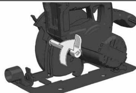
Adjust the cutting depth to the thickness of the workpiece. Less than a full tooth of the blade teeth should be visible below the workpiece.
