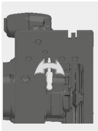
If a correction of the 90° angle of the guide-plate to the saw blade is necessary, use the correction screw.
